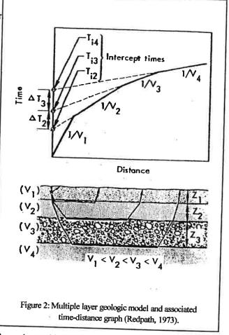
will not be refracted back to the surface until it encounters a deeper layer with a higher velocity, so no first arrivals are observed from the low-velocity layer. The presence of an unknown low-velocity layer will cause the calculated depths to be greater than the actual depths.
