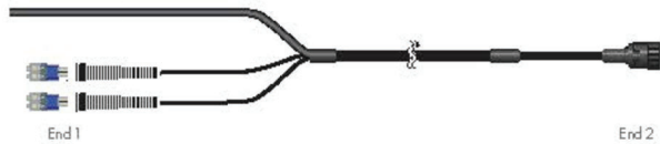
2 HYBRID JUMPER CABLE DETAIL SCALE: NTS
