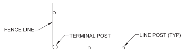
5 A-8 INSTALLATION AT CORNERS SCALE: NTS
