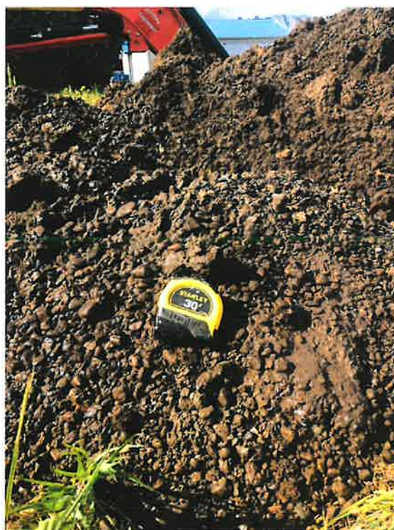
Coarse alluvium test pit spoils.
