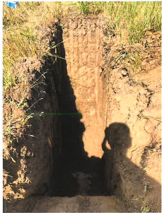
Completed test pit.
