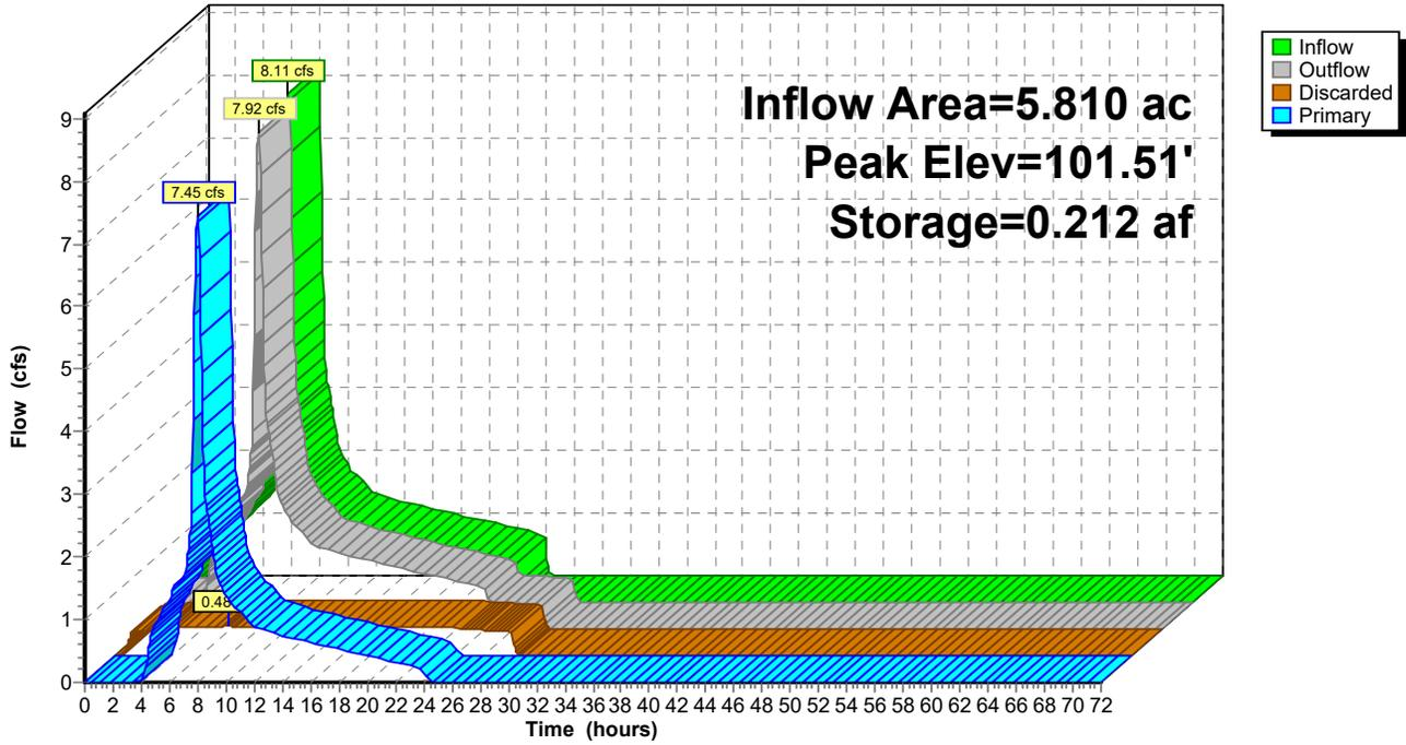
**S-1 Bioretention & Infiltration Ponds Connected**
