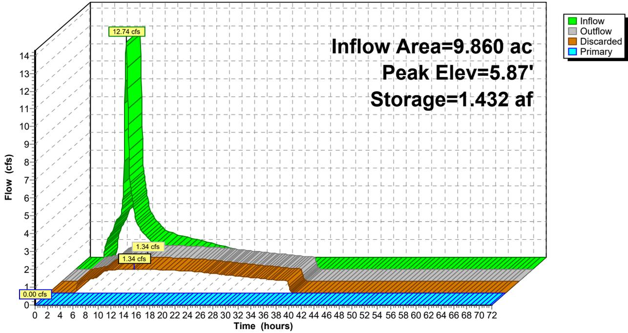
**S-1 Bioretention & Infiltration Ponds Connected**
