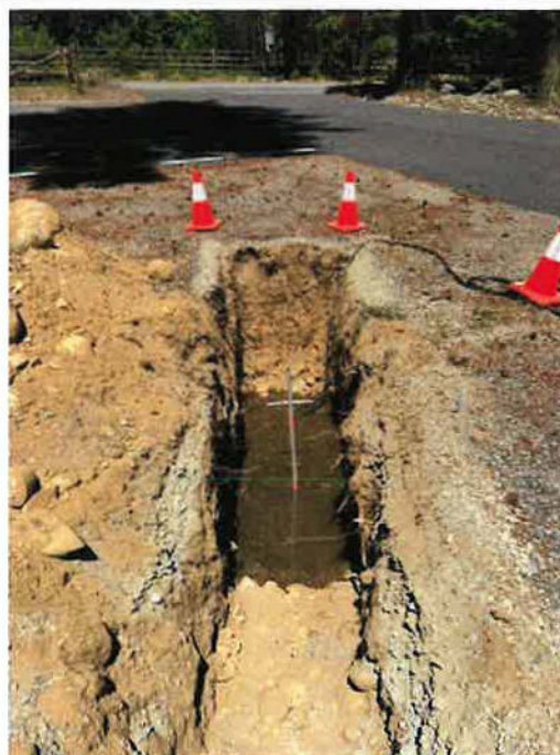
Left Photo: Tape measure at about 5 feet below grade. Right Photo: Infiltration test in progress.
